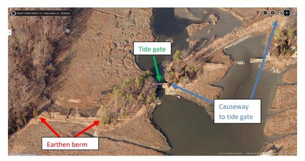
**Figure 3.** Aerial photograph of the Branford Trail where it crosses Jarvis Creek (from maps.bing.com; obtained between March-April 2011). On the eastern (right) side of the marsh the path is on a rock and earthen causeway (bounded by blue arrows) to the tide gate (green arrow). On the west (left) side of the marsh the trail crosses on to a timber bridge that was built above the location of the earthen berm that is indicated by the red arrows.
