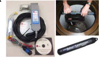
Clockwise from left: Doppler flow meter, Ultrasonic level sensor, and level logger
