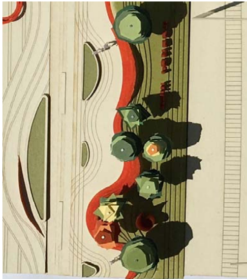
Landscape Solution Type A: A series of berms/landforms running between the train tracks and river. Will need a method (movable gates, etc.) to 'close' the ends of the berm system. This protects Amtrak, Water Street and buildings on eastside of Bank street from flood waters.
