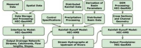
Figure 4: Flowchart of the distributed hydrologic and hydraulic modeling system for flood mapping [4].
