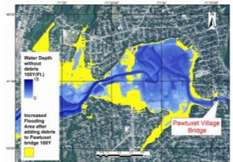
Figure 14: Effect of debris on the 100-yr flooding extent at the Pawtuxet Village bridge.
